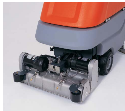
Low brush deck is ideal for cleaning underneath obstacles.
