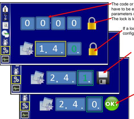
The code or diagnostic connector for setting parameters does not have to be entered or connected if the operator wants to adjust parameters (only released parameters can be adjusted).
