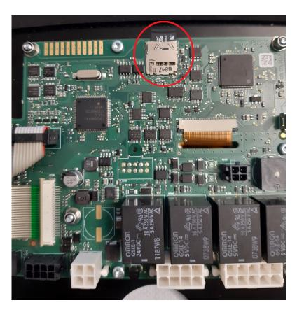
This picture indicates the position of the SD-card in the dash board.
