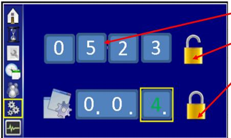
If parameters are to be changed, the code for setting parameters must be entered (alternatively, diagnostic connector).
